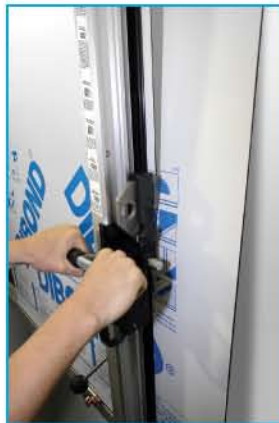
Cuts up to 4mm Dibond in one pass with clean finished edges.
