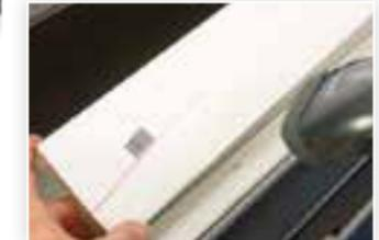
SCANNER READER IS AVAILABLE FOR READING SPECIFIC FORMATTED BARCODES OR QR CODES FOR LOADING AND SAVING PROGRAM IN CONTROLLER. (SOLD AS ACCESSORY ITEM)
